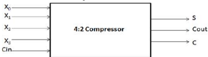
Figure-6: Block box of a 4:2 compressor adder
